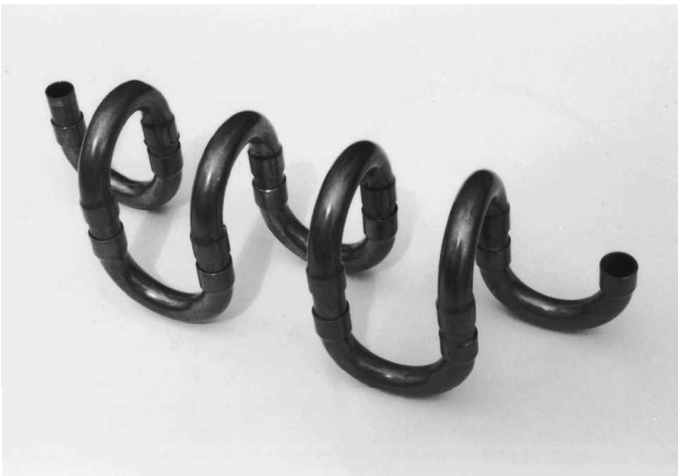
Fig. 9 Conventional coiled tube and alternating-axis tube.
