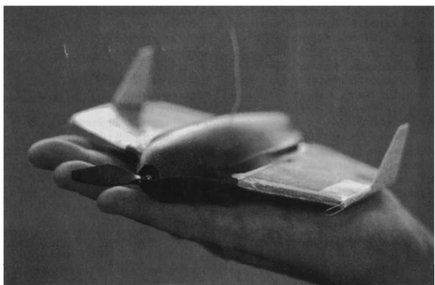
Fig. 2 Sanders MicroSTAR with 0.15-m wing span resting on a human hand.
