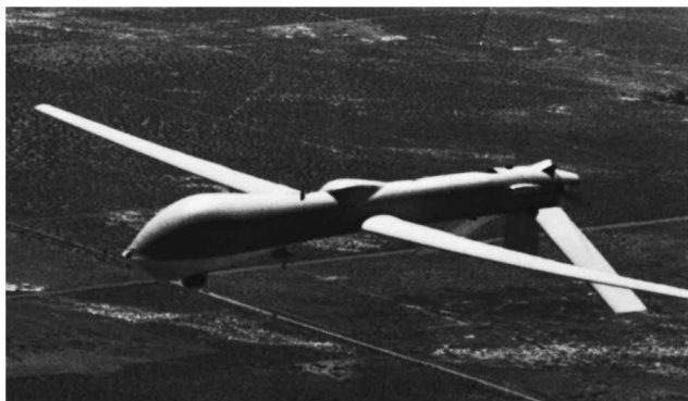
Fig. 1 Medium-altitude endurance UAV Predator with 14.8-m wing span.
